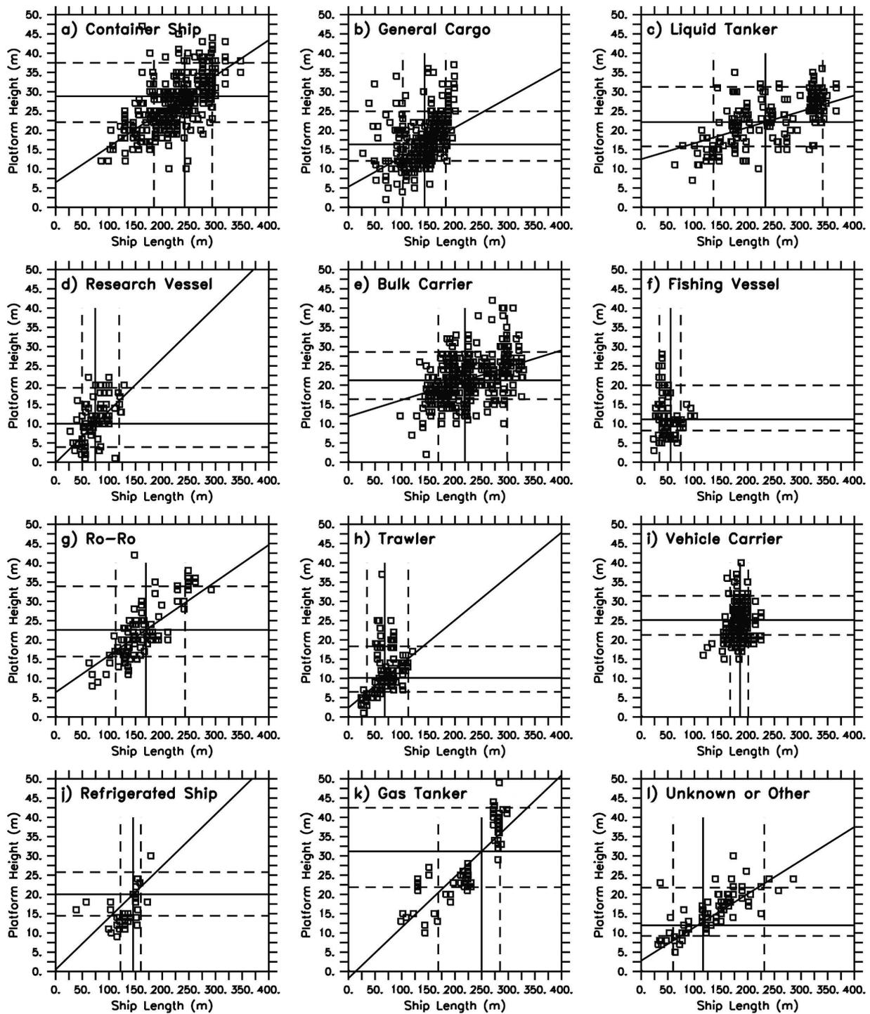
FIG. 8. Plots of platform height (m) against ship length (m) for the most commonly reporting different ship types. Horizontal and vertical solid lines indicate mean values, and dashed lines the 10th and 90th percentiles. The sloping solid lines indicate the results of linear regression.
