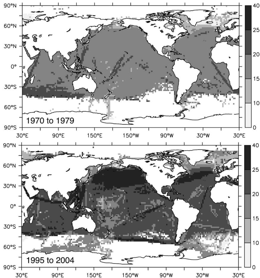
FIG. 4. The  $2^\circ$  area average air temperature measurement height (m) from Pub. 47 and ICOADS averaged over the periods (top) 1970–79 and (bottom) 1995–2004. Measurement height information is derived from different Pub. 47 metadata elements in different periods (platform height from 1970 to 1994, height of the barometer from 1995 to 2001, and air temperature measurement height from 2002 onward).
