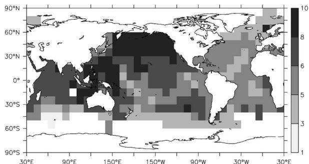
FIG. 12. The  $10^\circ$  area average SST measurement depth (m) from Pub. 47 and ICOADS for the period 1995–2004.
